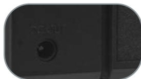
DC output for recharging both the FB-64 Belt Pack and FM-64 Handheld Microphone
